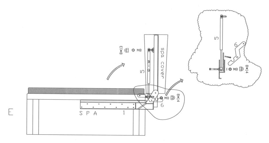
After lifting the insulation cover vertically Reinstall the air support rod
