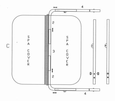
Two parts 4 are assembled separately on both sides of part 2
