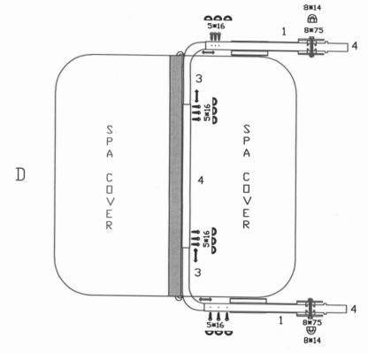
After selecting the appropriate position, fix it with screws, and select the screw cap as shown in the figure
