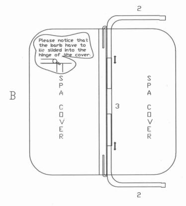
Part 3 and two parts 2are assembled on the insulation cover.
