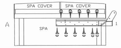
Fix part 1 on bpth sides of the spa with 5\*40 screws.
